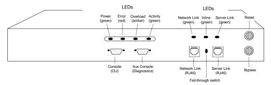
Figure A-1: Front Panel Connectors, Controls, and Indicators
